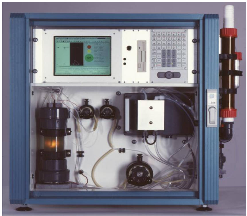
The new bbe Toximeter, an instrument with a wide detection range
