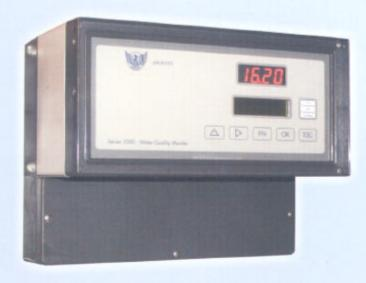
An IP65 microprocessor based instrument capable of measuring up to 5 different parameters together with alarm and retransmission facilities.
