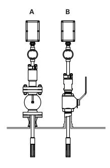
A: OWD<sup>®</sup> Insertable model installed on a main pipe with 2", 3", or 4" flanged seal housing **B**: KAM<sup>®</sup> OWD<sup>®</sup> Insertable installed on a main pipe with 2" MNPT seal housing
