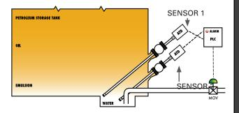
Two KAM® ATD sensors are inserted at an angle directly into the tank or from the top through full-opening ball valves.
